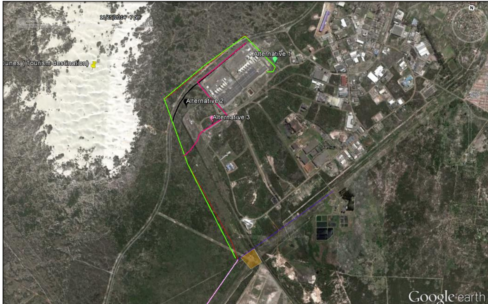
Figure 1 (b). Three alternatives proposed in November 2014 for the routing of the lines around the power station at Ankerlig. Alternative 1 (green) is the longest (5.1 km as shown) and occurs north of the Dassenberg Rd. Alternative 2 (black) is a short modification of that on the south of the road (4.0 km) and alternative 3 (pink) is around the substation (4.3 km) but is not considered feasible by Eskom for engineering reasons.
